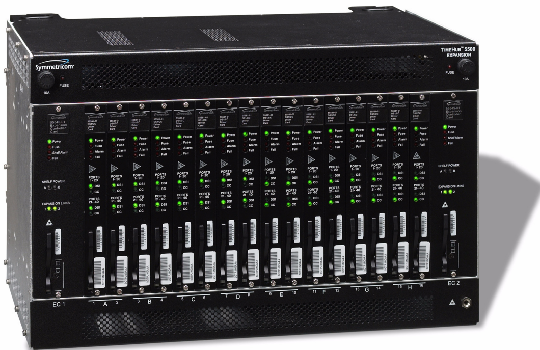
Figure 1-4. TimeHub 5500 Expansion Shelf – Front View
