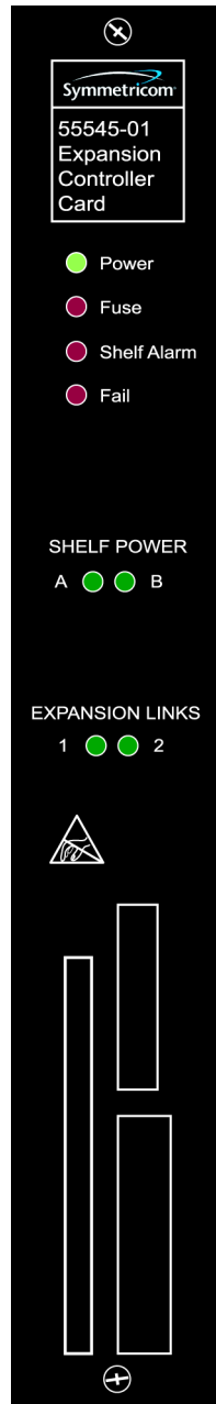
Figure 2-8. Front Panel of the Expansion Controller Card
